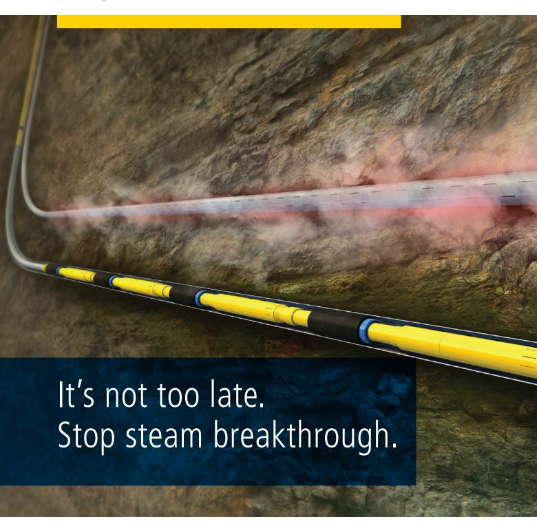
Avoid costly well re-completions and maximize ultimate recovery from existing SAGD wells with tubing-mounted, retrofitted flow control systems.
